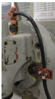
Electrical connectors attached to the head of the milling machine
