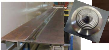
6m length butt weld in steel S355
